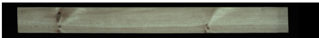
Figure 2. One-side photo of a wood veneer collected in a single run by the data acquisition equipment.
