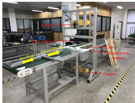
Figure 1. Acquisition equipment used to collect wood veneer images.
