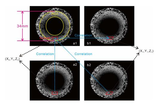
**Figure 7.** Principle of stereo matching of 3D-DIC images. (a1,a2) left image before and after deformation; (b1,b2) right image before and after deformation.
