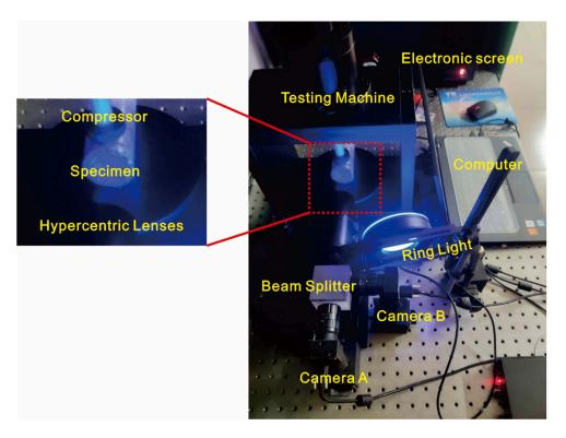
Figure 10. Pipeline compression test.
