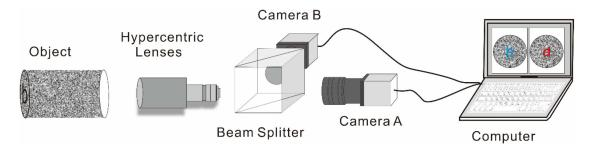
Figure 4. Schematic diagram of the coaxial dual camera with hypercentric lens.
