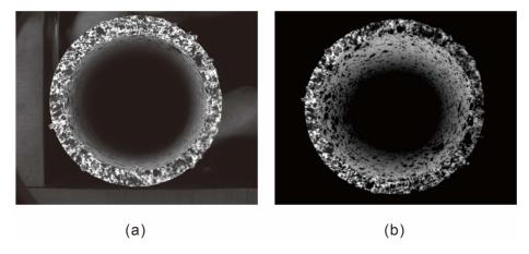
Figure 5. Comparison of field of view (a) without hypercentric lens and (b) with hypercentric lens.
