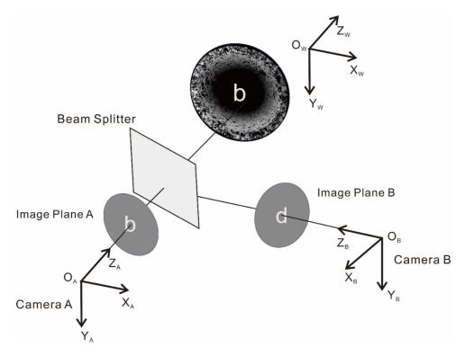
Figure 6. Schematic of binocular stereo visual effect of coaxial dual-camera system.
