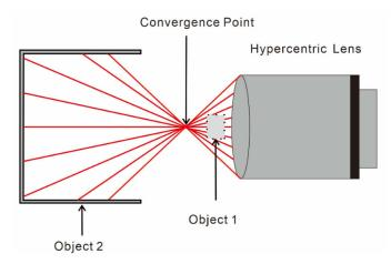
Figure 2. Principle of the hypercentric lens.
