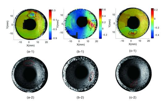
**Figure 13.** Strain distribution of defects at different positions: (a) upper part; (b) on the right side; (c) bottom.
