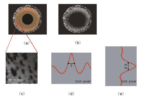
Figure 11. Collected images and speckle texture analysis: (a) image of camera A, (b) image of camera B, (c) typical areas of the subregion, (d) full width of horizontal half-peak, and (e) full width of vertical half-peak.
