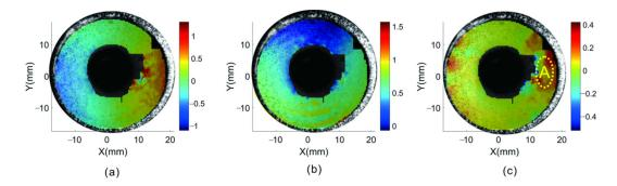
**Figure 12.** Pipe wall displacement and strain distribution under 10 kN load: (a) displacement of u-field; (b) displacement of v-field; (c)  $\varepsilon_{xx}$  strain.
