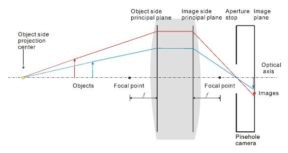
**Figure 3.** Model of a hypercentric lens.
