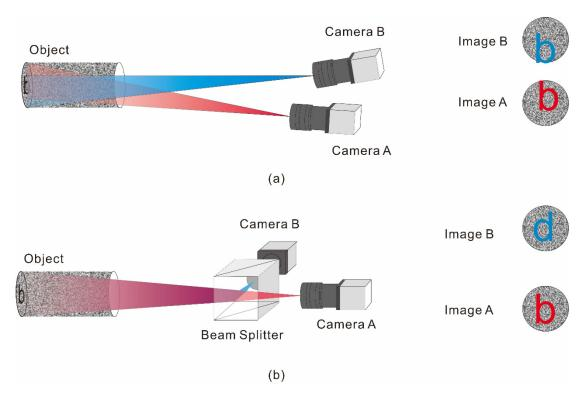
**Figure 1.** Optical path comparison. (a) Optical path of traditional dual-camera 3D measurement system; (b) Optical path of the coaxial dual-camera 3D measurement system.
