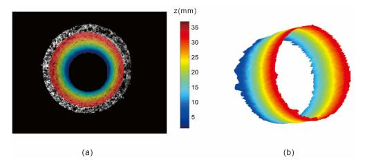
Figure 8. (a) Real calculation area; (b) Three-dimensional outline of the inner surface.
