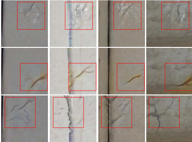
Figure 6. Illustration of spatial control in defect generation by Defect-GAN: Each row shows defect samples generated with different normal samples but the same spatial control, while each column shows defect samples generated with the same normal sample but different spatial controls.
