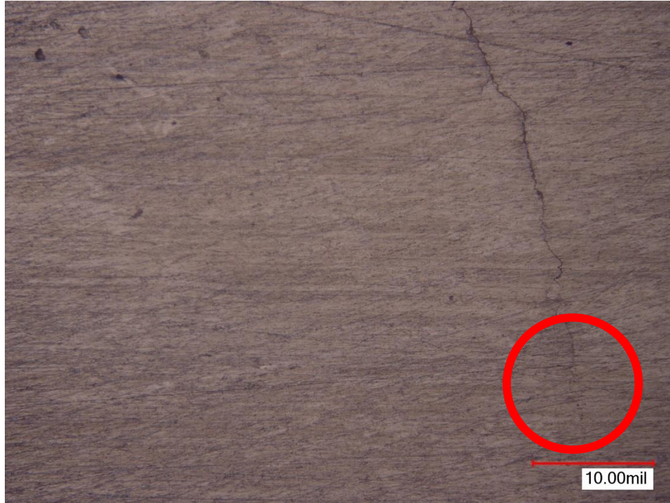
Figure 28: Specimen E1, external surface crack tip
