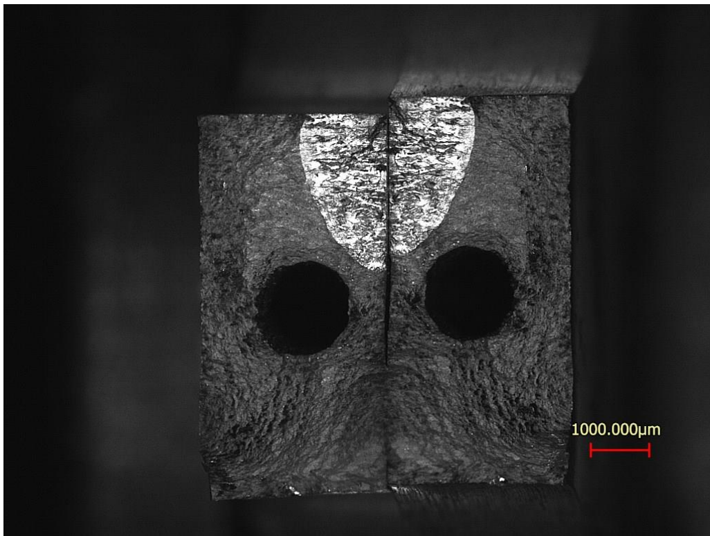
Figure 39: Specimen A3 fracture surface (10,000,000 cycles : 50.09 ksi / 345.3 MPa)
