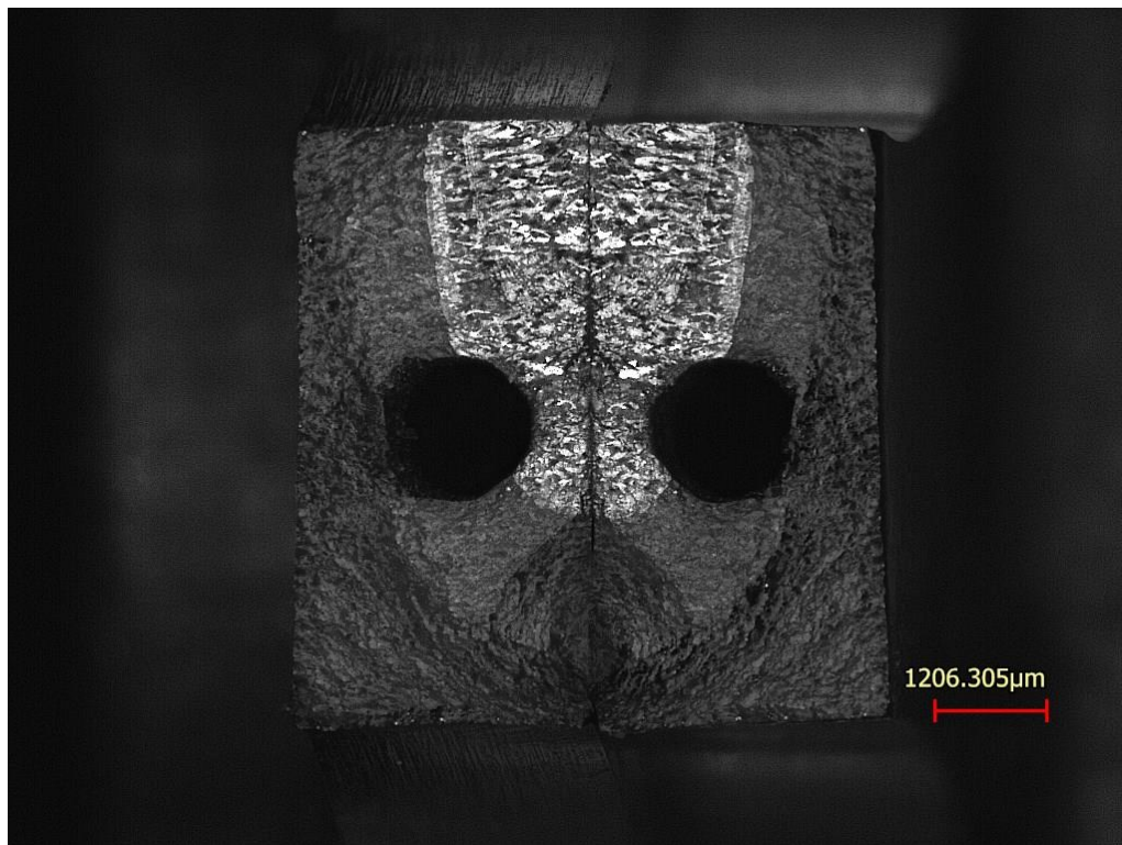
Figure 47: Specimen D2 fracture surface (3,000,000 cycles : 55.51 ksi / 382.7 MPa)
