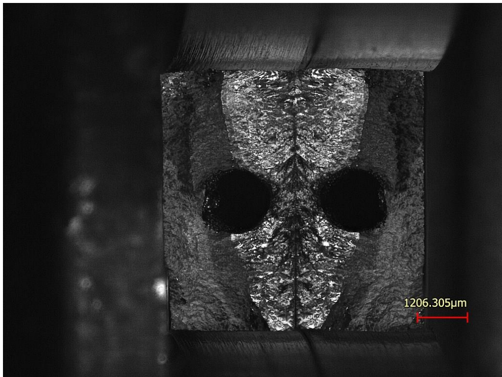
Figure 43: Specimen C1 fracture surface (1,000,000 cycles : 61.33 ksi / 422.8 MPa)
