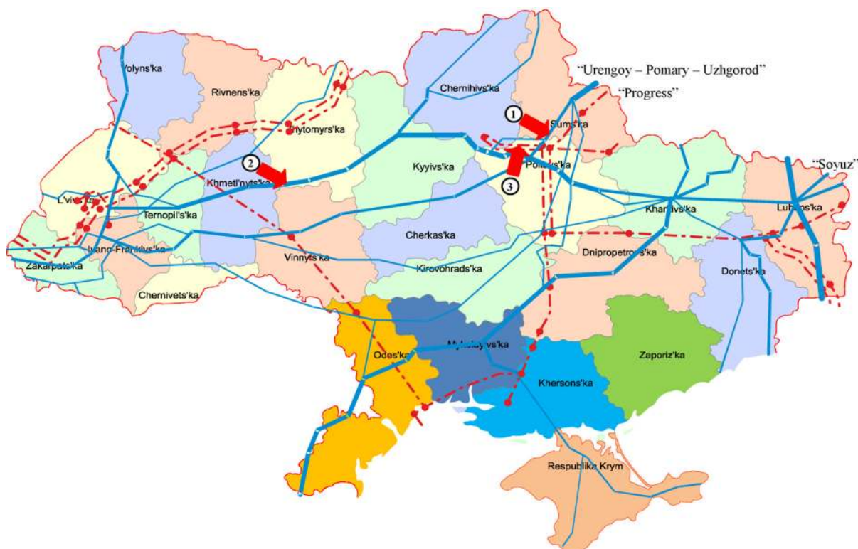
Fig. 1. Scheme of the Ukrainian main gas and oil pipelines (Voropai et al. 2012) and the steel billets of the investigated pipelines in the taking places (arrow marked): 1 – pipe branch “Mekhedivsko-Golotovshchinska Temporary Metering and Separation Station (TMSS)” of the main gas pipeline “Kursk–Kyiv”; 2 – main gas pipeline “Kyiv–West of Ukraine-1”; 3 – oil pipeline “Gnidyntsi–Glynsko–Rozbyshivska”
