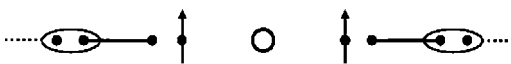
FIG. 11. The introduction of a nonmagnetic impurity in the spin-1 chain displayed in Fig. 6 breaks two singlet bonds, thereby releasing two spins 1/2 .
