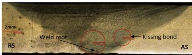
Fig. 5 Weld root and kissing bond in 6-mm FSW DH36 ( W_{2D} )
