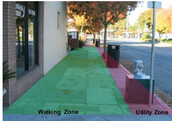
Figure 3. 4: Walking Zone and Utility Zone
