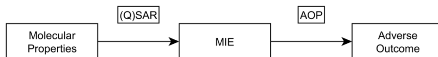
Figure 2. Framework for a (quantitative) structure activity relationship ((Q)SAR) approach based around MIEs. The (Q)SAR relates molecular properties to molecular initiating event (MIE), and the adverse outcome pathway (AOP) infers an adverse outcome from the MIE.
