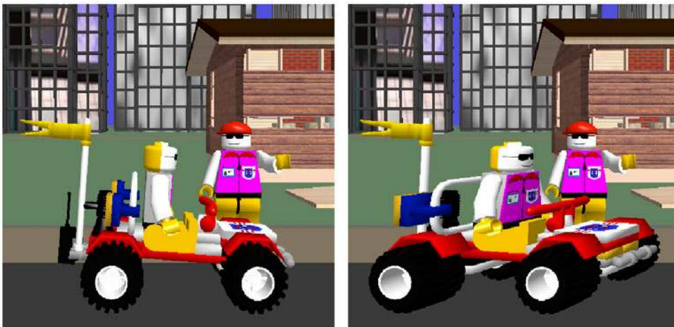
Figure 11. Single vs. multiple projections. The left image is a classic linear perspective view. The right image uses multiple projections, and each object is assigned a different drawing[spatial] system. The background house is depicted using linear perspective to convey a sensation of depth, while the car and foreground character are represented using oblique projection to enhance the visibility of the character's face. Image courtesy of Maneesh Agrawala.
