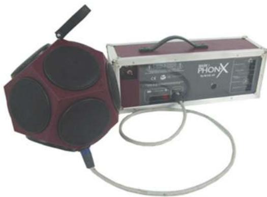
FIGURE 3: Dodecahedron FOUR and amplifier PHON-X Mark I.
