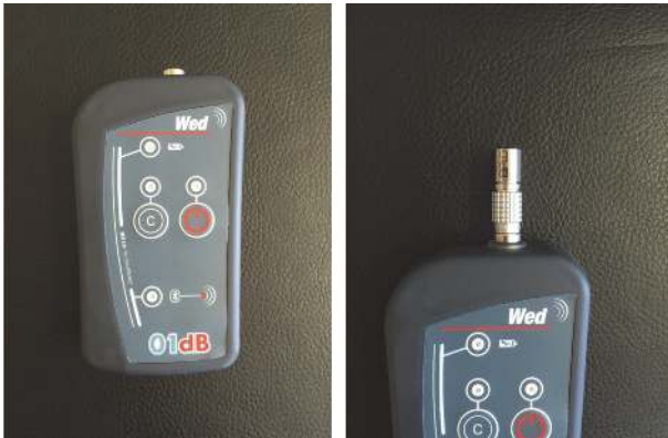
FIGURE 2: Noise dosimeter WED 007 with microphone, 01 dB.
