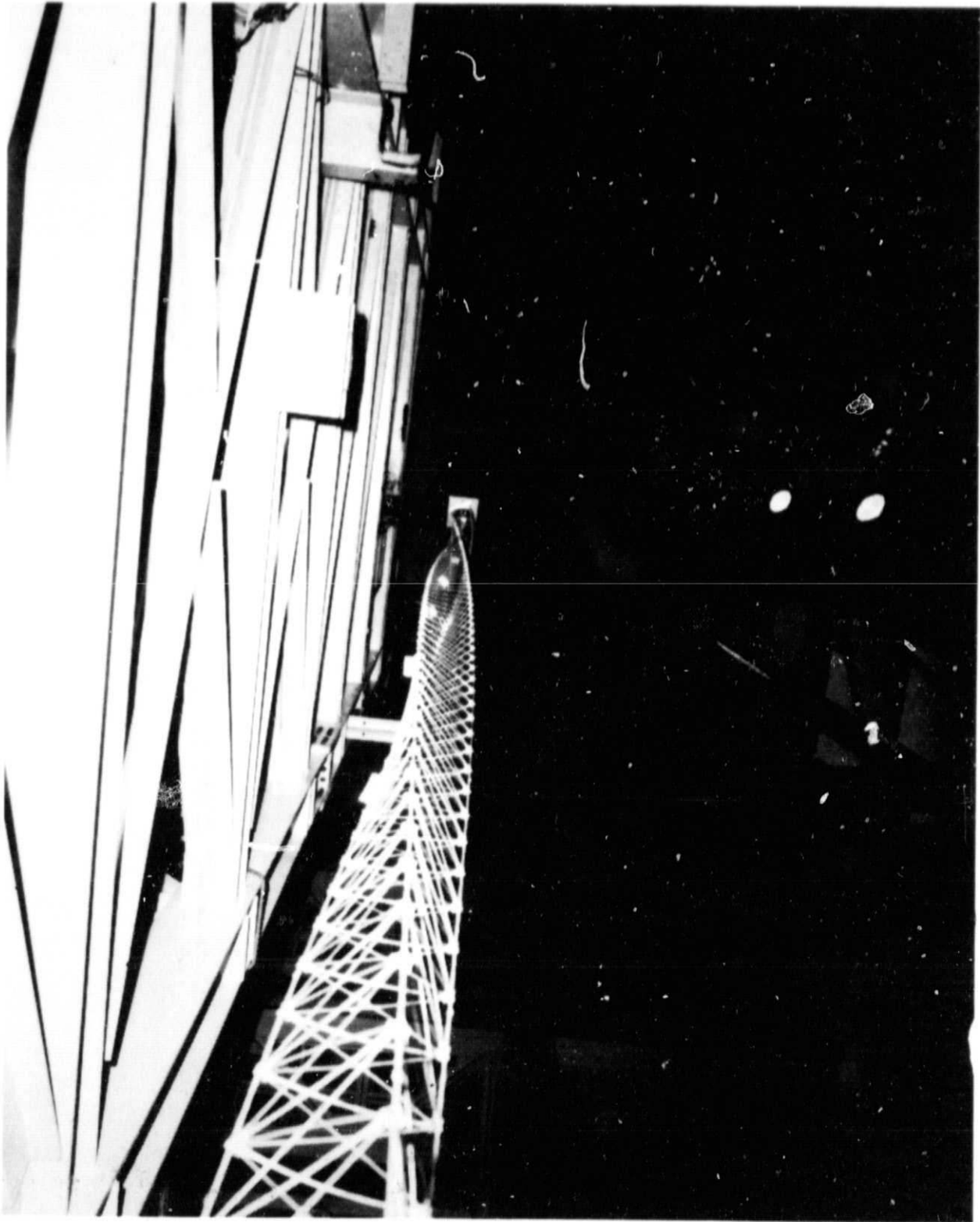
Figure 17. ASTROMAST beam showing 280 deg static twist about longitudinal axis.
