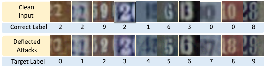
Figure 1: Deflected adversarial attacks on the SVHN dataset. These images were generated by a defense aware attack and the maximal adversarial perturbation is bounded by 16/255 .
