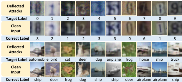
Figure 7: Deflected adversarial attacks on SVHN and CIFAR-10. The maximal \ell_\infty perturbation is 16/255 for SVHN and 25/255 for CIFAR-10.
