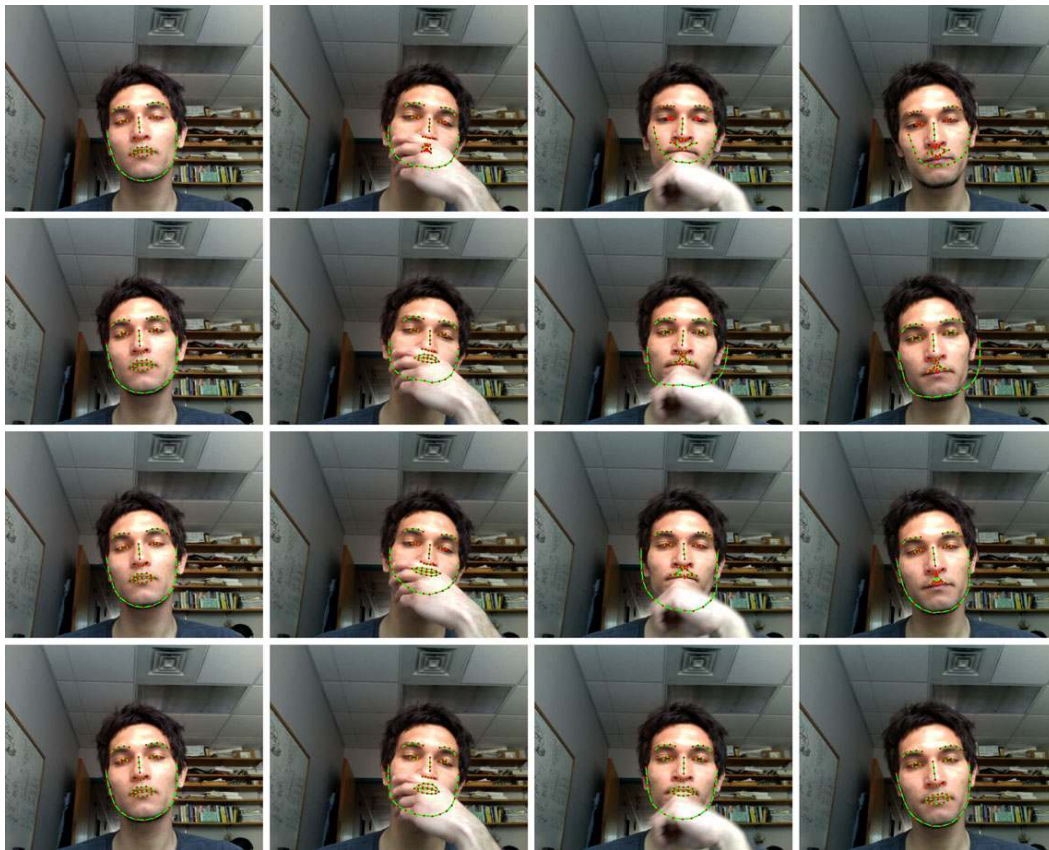
Fig. 8 Example of tracking with gross occlusion. Top to bottom rows: ML fitting with a Gaussian kernel, MAP fitting with a Gaussian kernel, ML fitting with a Geman-McClure kernel, and MAP fitting with a Geman-McClure kernel. Left to right columns: Frames 0, 30, 40 and 50
