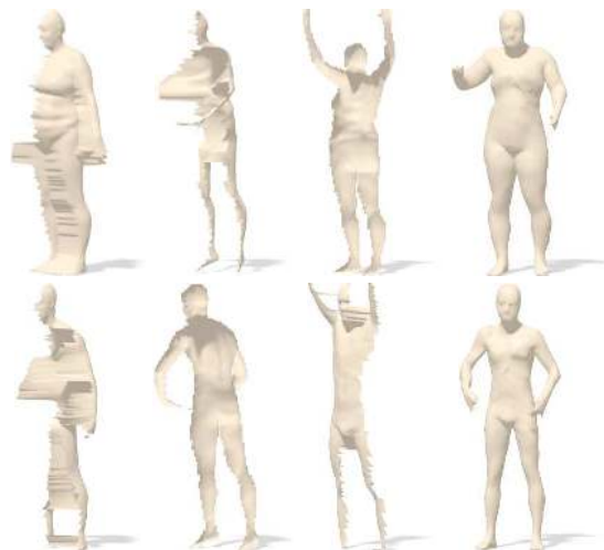
Figure 7. Dynamic fusion. Three partial views (columns 1-3) and the reconstructed complete shape (rightmost column).
