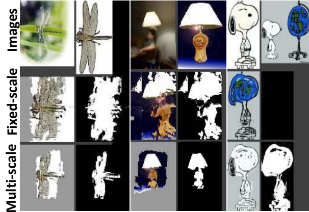
Figure 9. Example matching results by our multi-scale matching. For comparison, we also show results from our fixed-scale version. Our multi-scale method successfully finds the correct scale between objects, providing accurate matching. On the other hand, a single-scale one prefers the fixed size between objects, causing gross errors: e.g., in the 3rd example, Snoopy matches to a globe since they have similar size.
