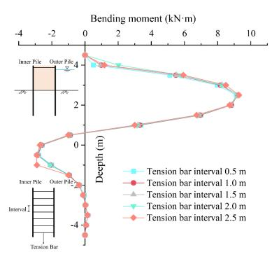
Figure 19. Pile bending moment of different tension bar interval conditions.
