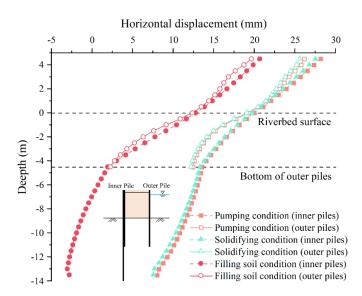
Figure 25. Horizontal displacement of reinforced piles.
