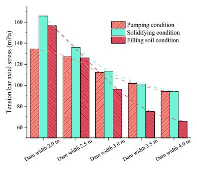
Figure 17. Tension bar axial stress of different dam width conditions.
