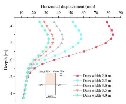
Figure 15. Pile horizontal displacement of different dam width conditions.
