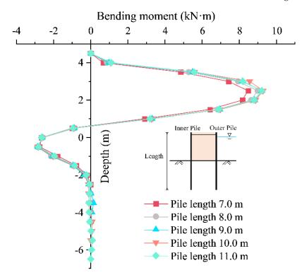
Figure 13. Pile bending moment of different pile length conditions.
