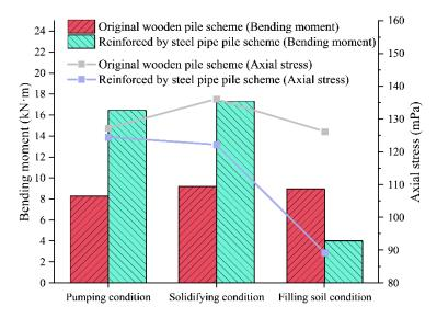
Figure 27. CoMParison of the internal force between reinforced piles and double-row wood piles.
