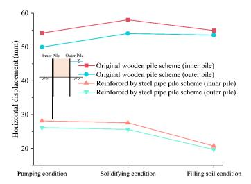
**Figure 26.** CoMParison of the horizontal displacement between reinforced piles and double-row wood piles.
