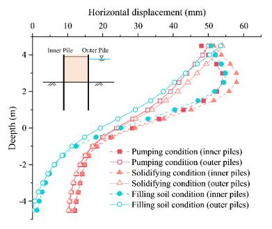
Figure 10. Horizontal displacement curve of piles at different stages.
