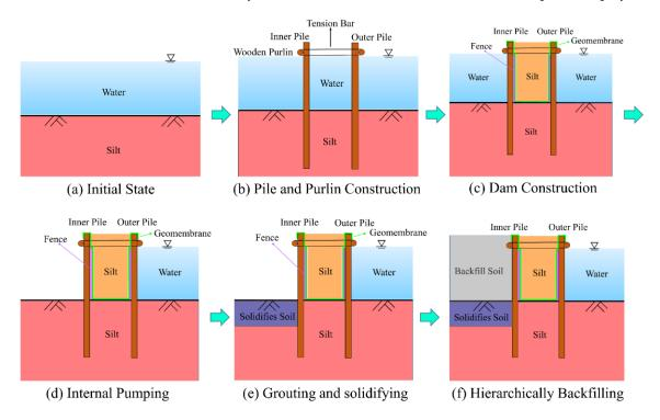
Figure 7. Construction steps.
