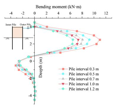
Figure 22. Pile bending moment of wood pile interval conditions.
