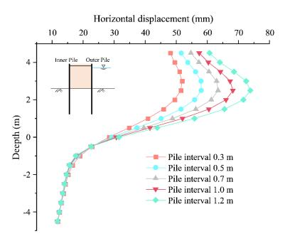
Figure 21. Pile horizontal displacement of wood pile interval conditions.
