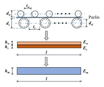
Figure 4. Equivalent of a combination of steel pipe piles and wood piles.
