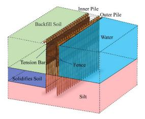
Figure 6. Double row wood pile structure.
