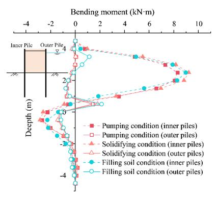
Figure 11. Bending moment of piles at different stages.
