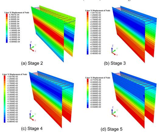
Figure 9. Horizontal displacement contours of piles at different stages (unit: m).
