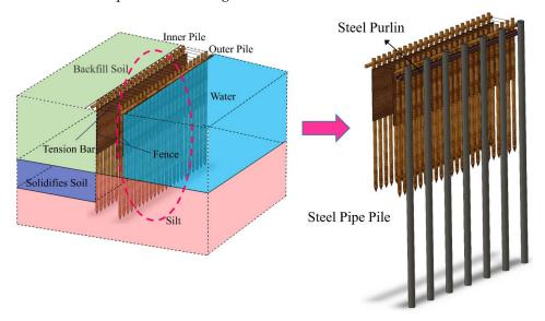
Figure 24. Steel pipe pile reinforced cofferdam structure.
