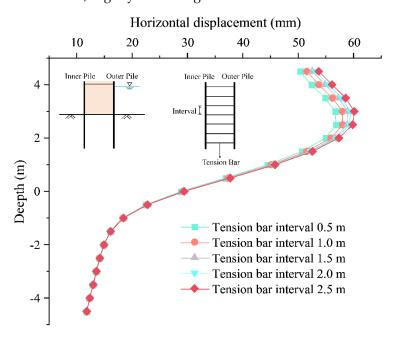
Figure 18. Pile horizontal displacement of different tension bar interval conditions.
