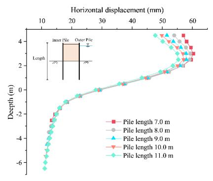
Figure 12. Pile horizontal displacement of different pile length conditions.
