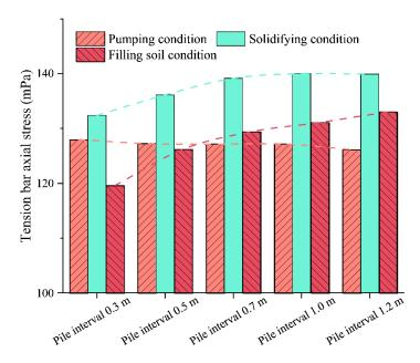
Figure 23. Tension bar axial stress of wood pile interval conditions.
