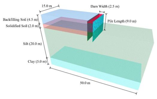
Figure 8. Mesh of the numerical model.
