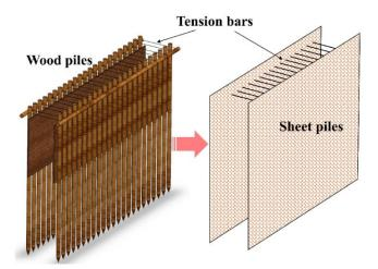
Figure 1. Equivalence of cofferdam structure.
