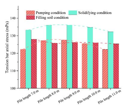
Figure 14. Tension bar axial stress of different pile length conditions.
