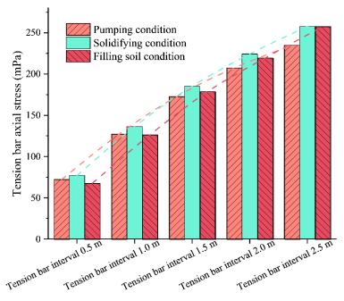
Figure 20. Tension bar axial stress of its different interval conditions.
