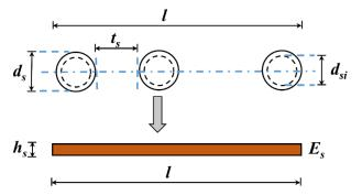
Figure 3. Equivalent of steel pipe piles.
