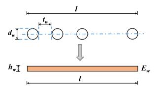
Figure 2. Equivalent of wood piles.
