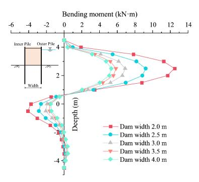
Figure 16. Pile bending moment of different dam width conditions.
