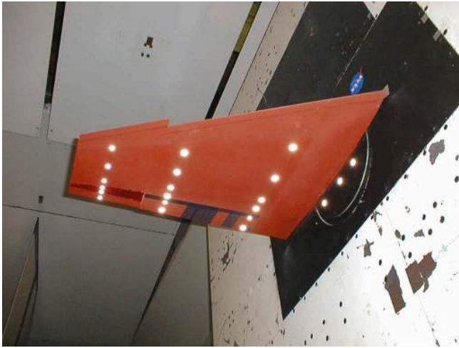
Figure 1: NGC Smart Wing with VMD targets at 22.7-, 61.2-, and 85.6-percent span.
