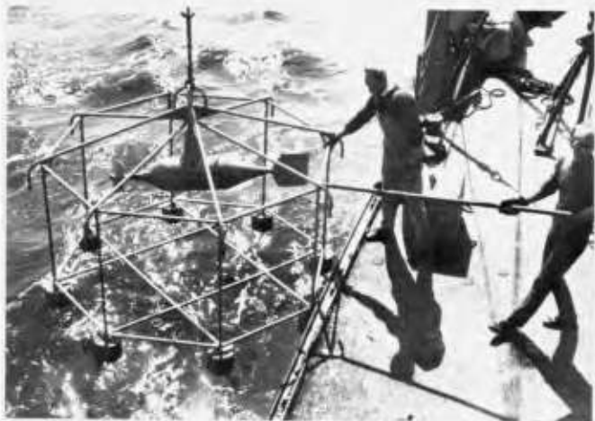
Fig. 11 Recording current meter for use in shallow coastal water
