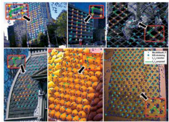
Fig. 9. Phase I results: The green L-shape inside the red enlarged rectangular window is the proposed (t_1, t_2) vector pair, and the red L-shapes are its supporting members (inlier votes). The images are cropped to emphasize the area of interest.
