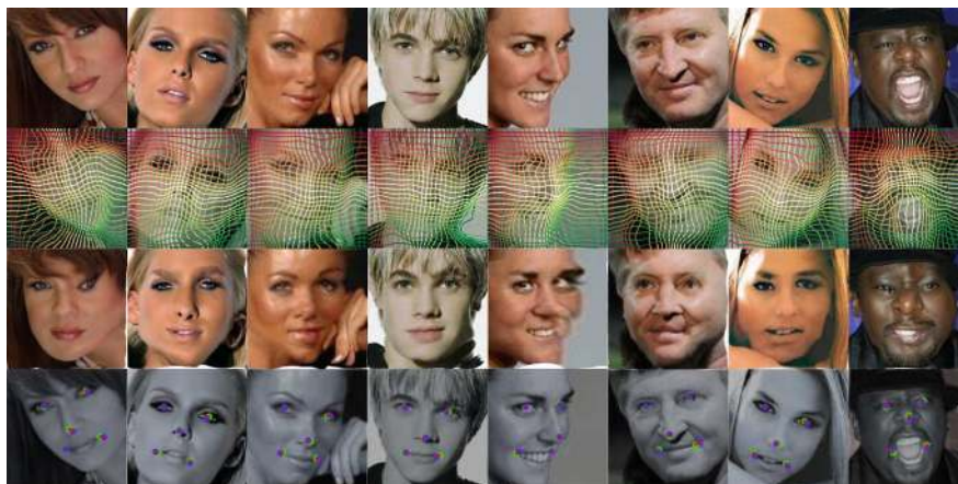
Fig. 12. Row 1: testing images; row 2: estimated deformation grid; row 3: image reverse-transformed to texture space ; row 4: semantic landmark locations (green: ground truth, blue: estimation, red: error).
