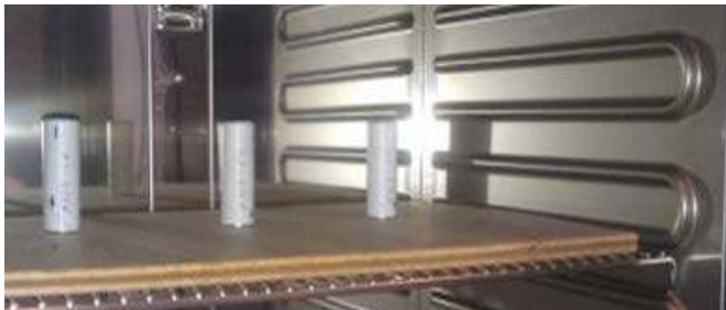
Fig. 1. LFP/C battery cells during accelerated calendar ageing tests.
