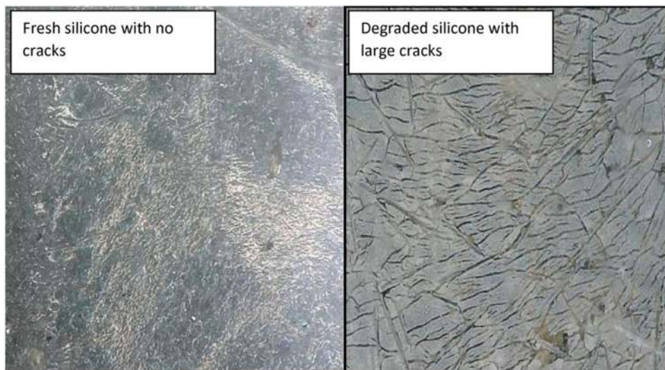
Figure 16. Cracks in the silicone after degradation [185], reproduced with permission from Elsevier.
