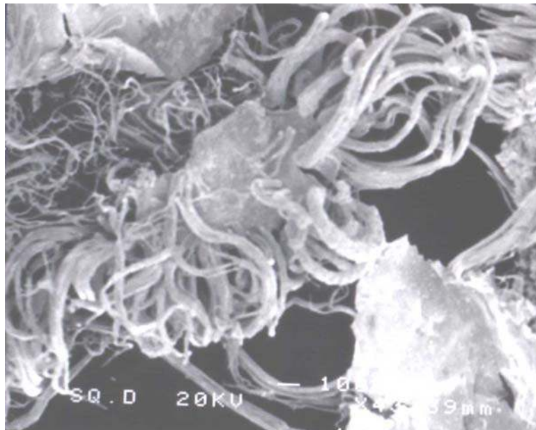
Fig. 12. Whiskers growing from the flakes, x43
