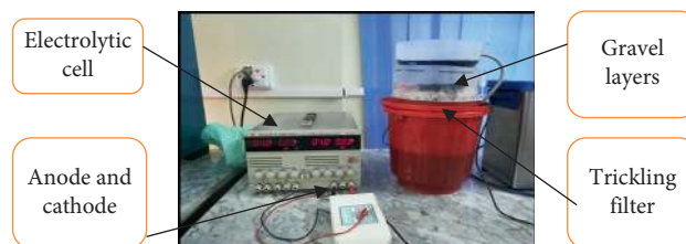
FIGURE 3: Trickling filter. It consists of gravels layer, electrolytic cell, and anode and cathode.
