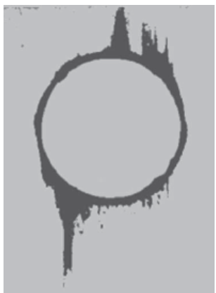
Figure 7 – Example of processing a radiographic image: (a) original image, (b) image segmented by using a neuronal network, (c) identified delamination region [20].
