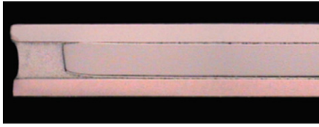
Figure 7. Optical image of the cross section of a copper laminated MOD-RABiTS tape, where both 50 \mu\text{m} thick copper laminates extend over the edges of the 75 \mu\text{m} thick slit coated conductor (sample 5 in table 1). One solder fillet is visible on the left of the image (only part of the cross section with one conductor edge is shown). Figure courtesy of American Superconductor Corporation.
