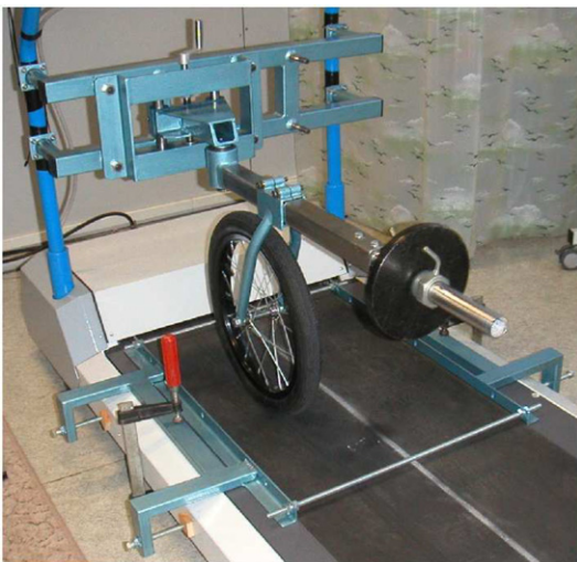
Fig. 6. The experimental rig on the stiffened conveyor belt.
