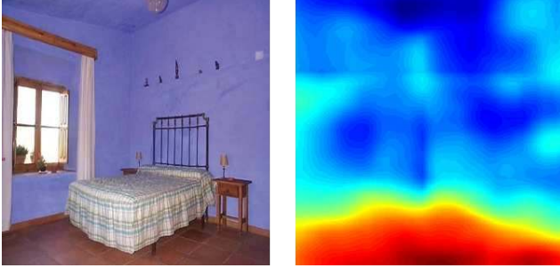
Figure 2: Given a w \times h \times 3 input RGB image (shown on the left), our neural network outputs a w \times h \times 5 belief map, where each of the 5 slices can be interpreted as a classification map for a specific label. For instance, the slice shown on the right corresponds to the ground plane label.
