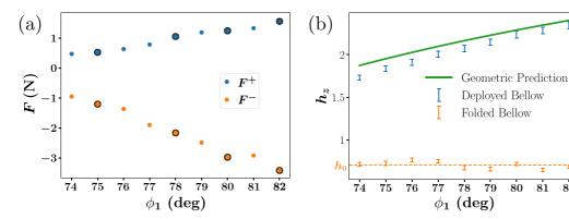
FIG. 4. (a) Force thresholds with respect to the pattern angle  $\phi_1$ . The four highlighted modules are those used in Sec. III B. (b) Normalized height  $h_z = \frac{H_z}{\ell_1}$  measured for the folded and deployed configurations. The solid green line corresponds to the geometrical prediction of the deployed height given by (3). The dashed orange line corresponds to the mean value  $h_0 = 0.70$  measured for the folded height.
