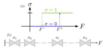
FIG. 5. Schematic description of the Preisach model. (a) Transition cycle for a hysteron  $\sigma$ , an element with two stable configurations 1 and 0, with respect to the external loading F.  $F^+$  ( $F^-$ ) is the loading threshold for the 0  $\rightarrow$  1 (1  $\rightarrow$  0) transition. (b) Stack of L independent hysterons  $\sigma_i$  in series symbolizing a stack of modules.
