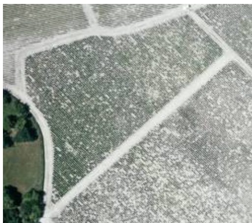
Figure 1. Typical high resolution remote sensed image of a vineyard. The resolution is 0.15m per pixel, the image size is 1825×1609 pixels i.e. approximately 274 m x 241 m.
