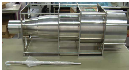
Fig. 4 8 mode horn for Shanghai 25m radio telescope.
