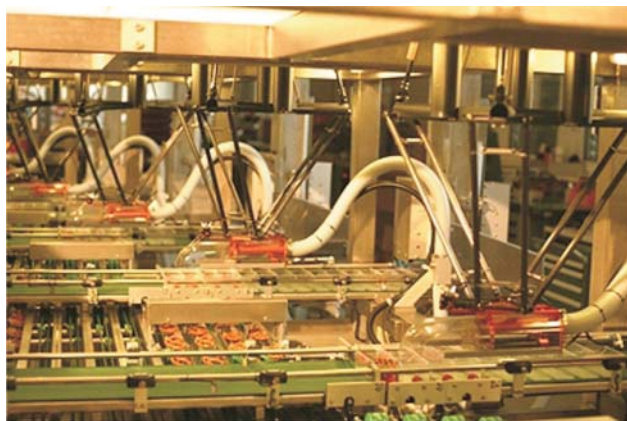
Figure 8 Demareux's Line-Placer installation for the packaging in an industrial bakery [9]
