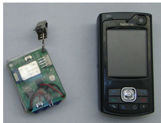
Figure 3: Our prototype key ring sensor attachment provides a GPS receiver and a 3-axis accelerometer.
