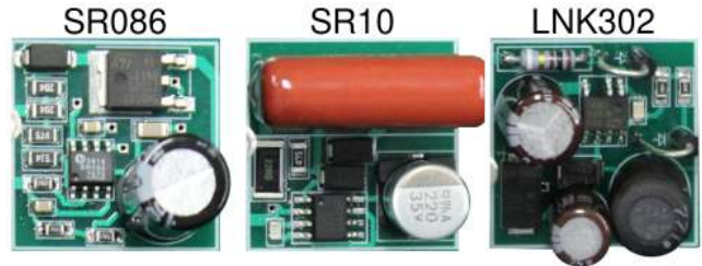
Figure 4: Low volume power supplies. Each supply is built within a 0.875 inch square. Large volume components are necessary for each supply and cannot be reduced significantly as load power decreases.
