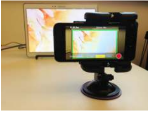
Figure 9: Experimental setup with Samsung Tab S (left) as the transmitter and iPhone 5s as the receiver (right).
