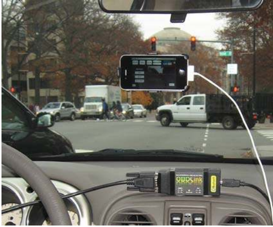
Figure 2: SignalGuru-enabled iPhone mounted on the windshield. The OBD-LINK device used to measure fuel consumption is also shown.
