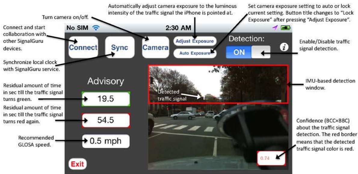
Figure 6: SignalGuru service screenshot. GLOSA advisory has also been included in the same iPhone application. Audio advisory can complement the visual advisory to alleviate driver distraction.
