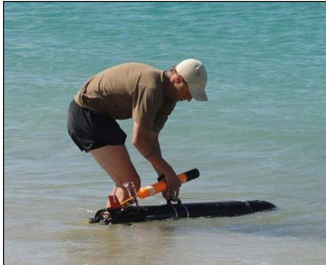
Fig. 1 (a-c) The NRP Bacamarte. Of Marinha Portuguesa provided services as served as a transport and launch platform for AUVs during REP 10A. The AUVs were launched while underway at 5 kts from the vessel quarter using a canvas sling. Approximately 2 minutes were available between sequential launch points to prepare and deploy the AUVs. Shore launch of multiple vehicles was easily accomplished in 0.5 m of water depth using a delayed launch, with a total launch sequence of < 2 minutes.
