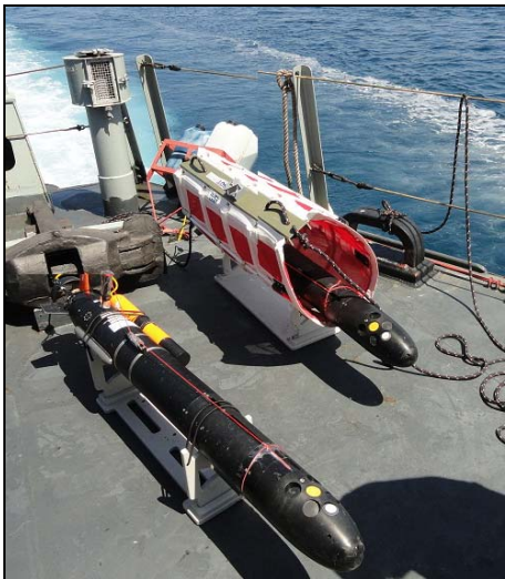
Fig. 1 (a-c) The NRP Bacamarte. Of Marinha Portuguesa provided services as served as a transport and launch platform for AUVs during REP 10A. The AUVs were launched while underway at 5 kts from the vessel quarter using a canvas sling. Approximately 2 minutes were available between sequential launch points to prepare and deploy the AUVs. Shore launch of multiple vehicles was easily accomplished in 0.5 m of water depth using a delayed launch, with a total launch sequence of < 2 minutes.
