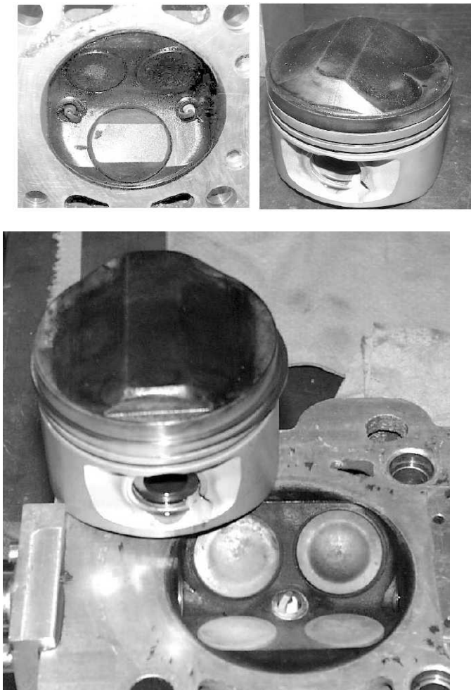
Figure 8. Top: Alvar engine cylinder head without the cover and camshaft mounted. Middle: Alvar engine combustion chamber and piston. Bottom: Standard engine combustion chamber and high compression piston.
