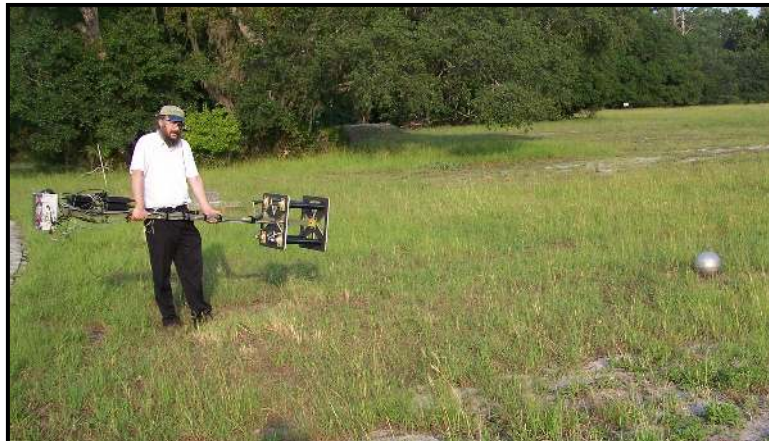
Fig. 3. Man-portable STAR Gradiometer being carried in the vicinity of a simulated target (a 31-cm steel sphere). The black boxes near the Operator's right hand are commercial analog to digital converter (ADC) units. The white box contains the sensor system's CPU, batteries and GPS receiver. The heads-up display unit (not easily visible in the unmagnified photo) is clipped onto the Operator's safety glasses.
