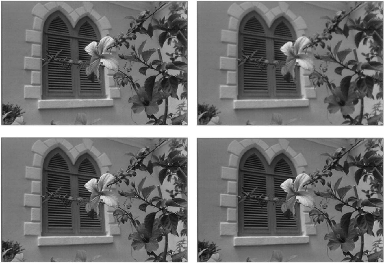
Fig. 6. Top left: original window image. Top right: result of a bilinear interpolation for the missing points for each channel. Bottom left: result of the first reconstruction by weighted interpolation step. Bottom right: second step enhancement result. This figure can be seen in color at www.cs.technion.ac.il/~ron/demosaic.html .
