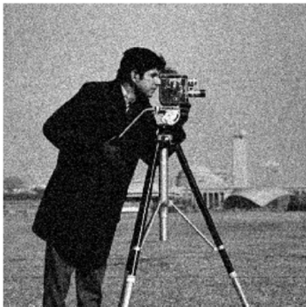
Image 4.1: Image corrupted with Gaussian noise, variance 0.005
