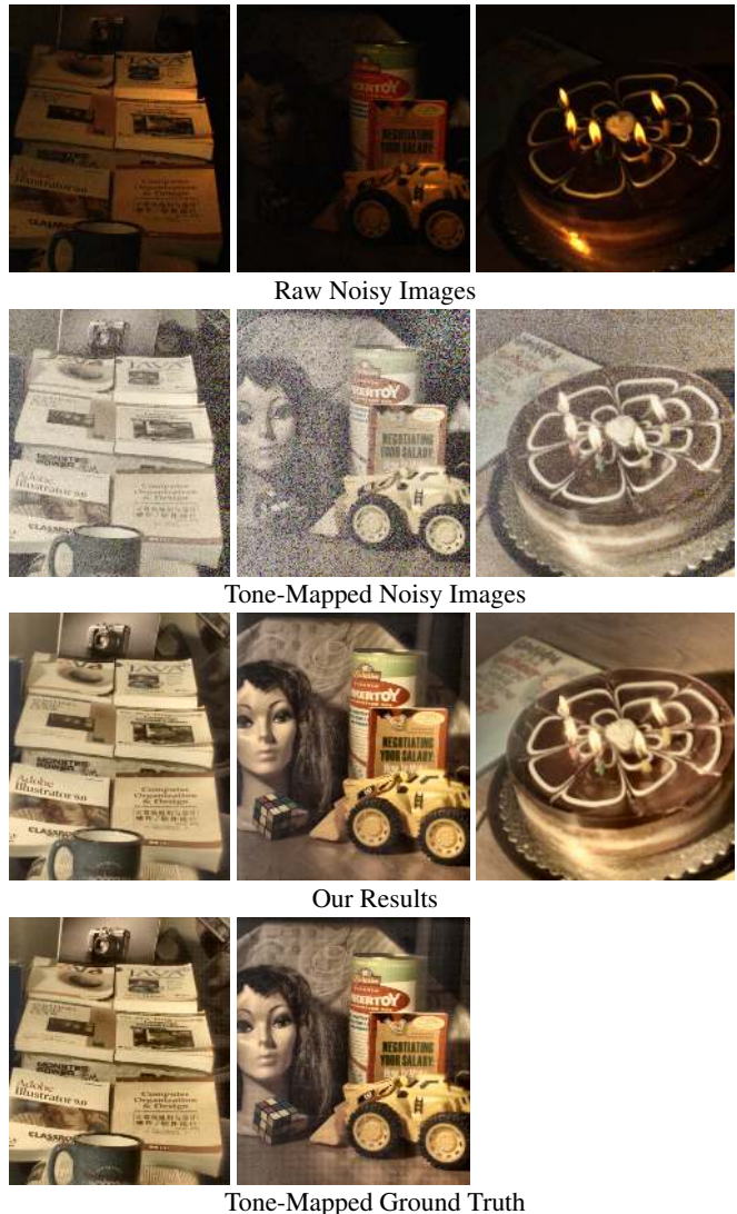
Figure 4. Computing HDR images from a sequence of 100 noisy images captured by a 14-bit handheld moving camera for three different scenes. The noise in the input images is higher in dark regions, as shown in the tone-mapped images. Our approach produces sharp and clean HDR images, and works for complex scenes with large depth variation. The cake scene has dynamic flames, and therefore does not have a ground truth. Best viewed electronically.
