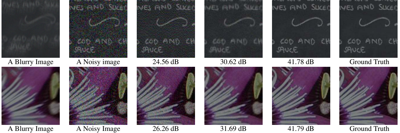
Figure 1. A comparison between single-image deblurring and multi-image denoising. From left to right: A blurry image B , \sigma_b = 2 ; One of the 100 noisy images, \sigma_n = 20 ; Deblurring using Eq. (18) as a weak prior; Deblurring using Eq. (19) as a stronger prior; Denoising using Eq. (18) as a weak prior. Even with a weak prior, multi-image denoising performs much better than single-image deblurring with a stronger prior. Please refer to our supplemental material for full resolution results. Best viewed electronically.
