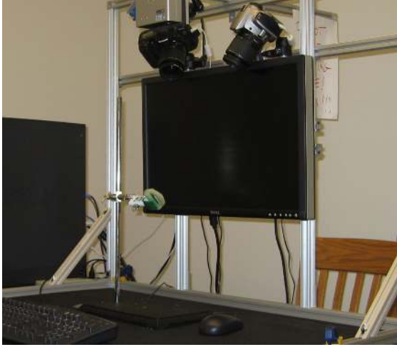
Figure 5. Photograph of our experimental setup. The object is placed in front of the monitor, facing the camera pair. The cameras capture image pairs while the monitor displays sweeping linear light sources. The small projector visible above the cameras is used for comparison with structured-light reconstructions.
