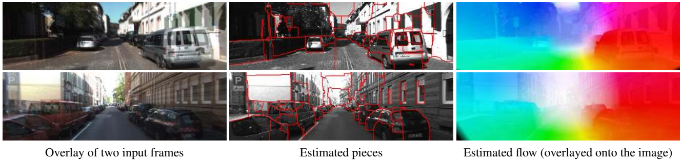
Figure 4: Example results of our method on KITTI benchmark. Note that in the example of the first row, motions of small objects such as the road lamp and sign are successfully estimated (flow color scheme of the benchmark is used).
