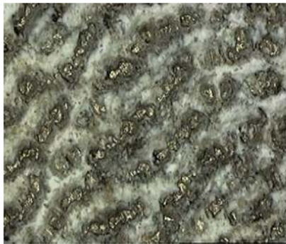
Fig. 10 Discontinuous powder melting between adjacent tracks (reproduced with permission from Ref. [76], © the Editorial Council for The Journal of Prosthetic Dentistry 2018).
