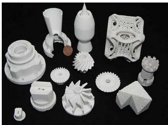
Fig. 6 Pure alumina parts processed by SLM (reproduced with permission from Ref. [55], © Materials Research Society 2014).
