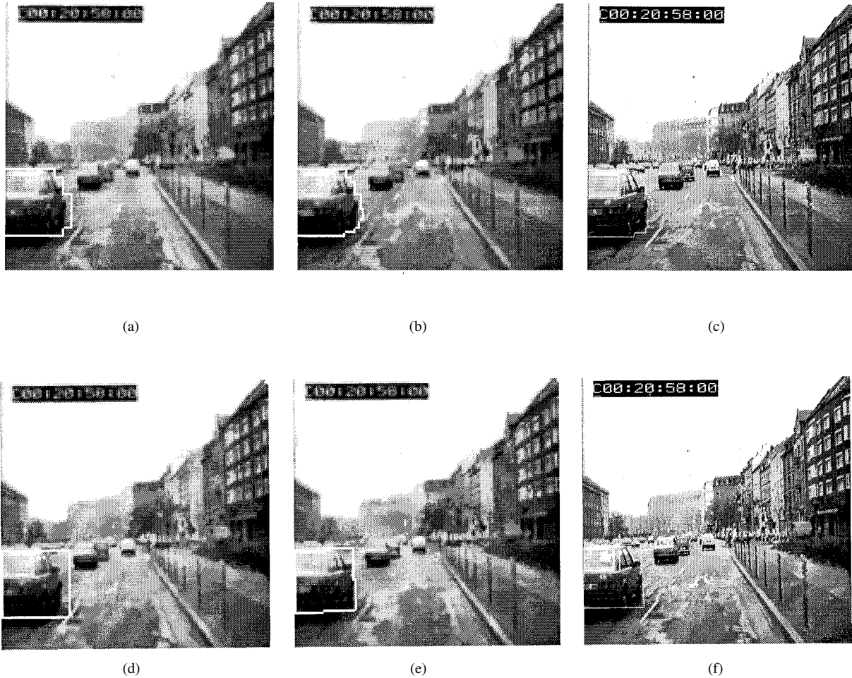
Fig. 13. Single object motion segmentation on street: (a)–(c) with an unconstrained closed curve , in \Omega^{2,2} , \Omega^2 , and \Omega , and (d)–(f) with a convex quadrilateral in \Omega^{2,2} , \Omega^2 , and \Omega .
