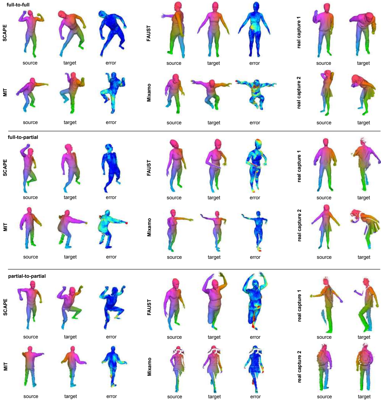
Figure 5: Our system can handle full-to-full, partial-to-full, and partial-to-partial matchings between full 3D models and partial scans generated from a single depth map. We evaluate our method on various real and synthetic datasets. In addition to correspondence colorizations for the source and target, we visualize the error relative to the synthetic ground truth.
