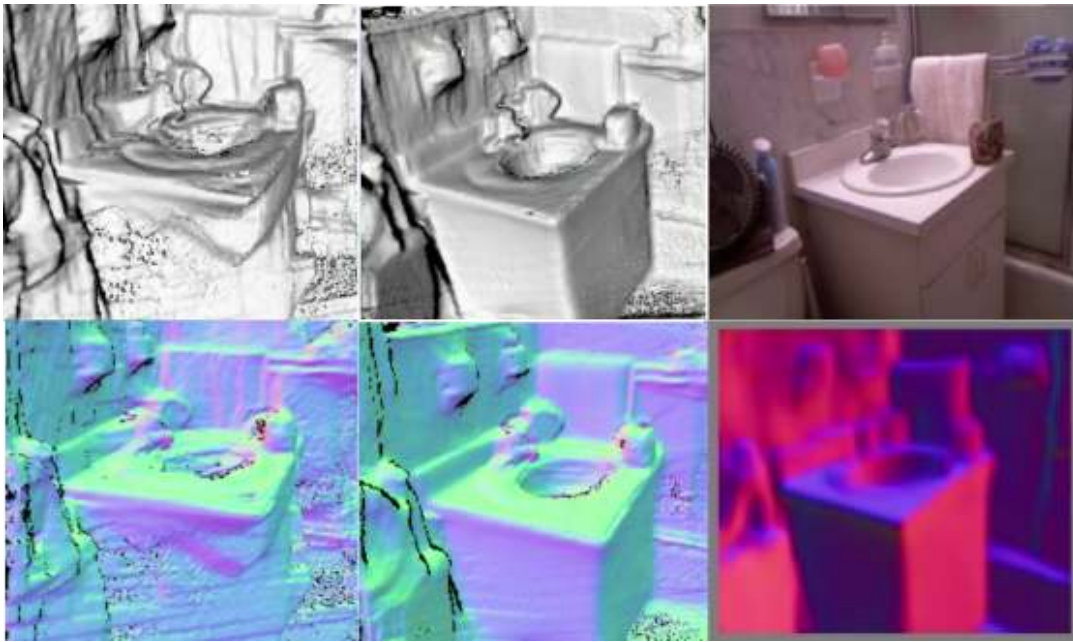
Fig. 5. Qualitative results on NYU raw dataset 'bathroom_0003' test sequence. Phong shaded fused reconstruction using smoothness prior (top left), phong shaded fused reconstruction using normals prior (top middle), a rgb keyframe image in the sequence (top right), surface normal rendering of fused smoothness-prior reconstruction (bottom left), surface normal rendering of fused normal-prior reconstruction (bottom middle), corresponding normal predictions for rgb keyframe image (bottom right). Note the more accurate reconstruction of textureless regions like the inside of the round sink using the normal-prior. A live comparison video is available at https://youtu.be/BRLN-1MTZtw .
