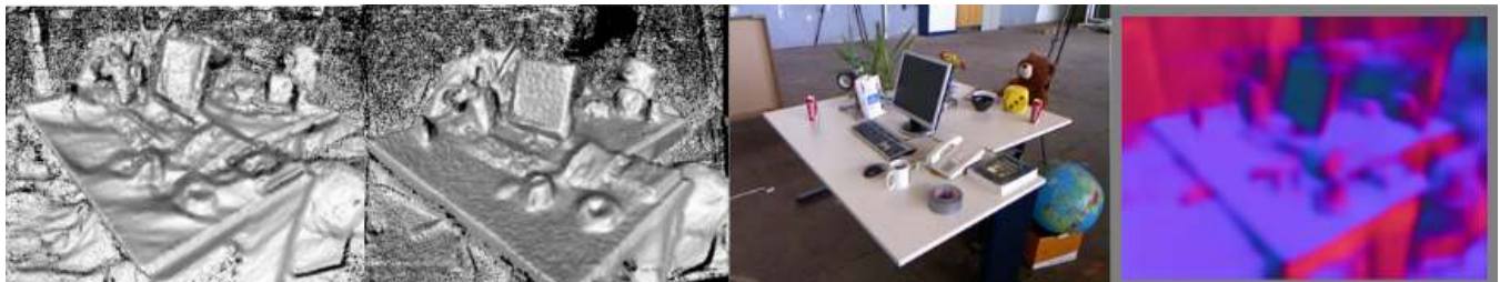
Fig. 7. Qualitative results on TUM dataset 'fr2_desk' sequence. From left-to-right are fused reconstruction using smoothness prior, fused reconstruction using normals prior, a rgb keyframe image in the sequence, and corresponding normal predictions for rgb keyframe image.
