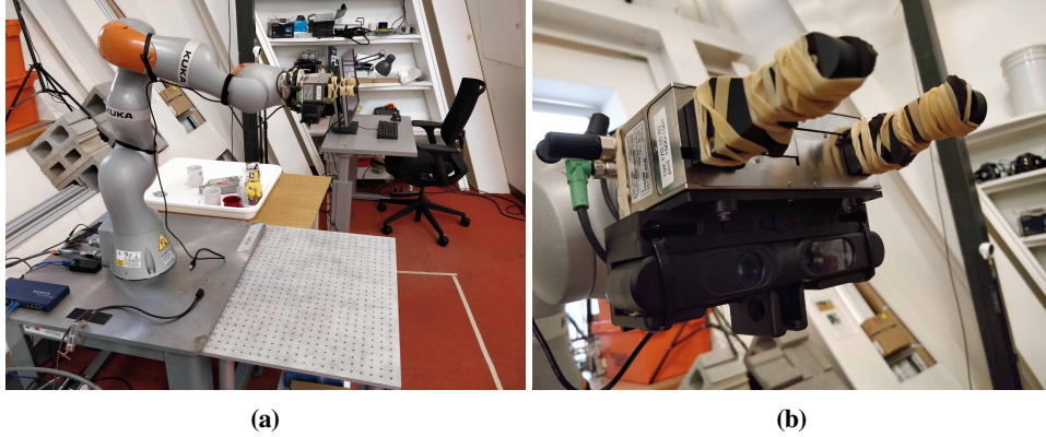
Figure 7: (a) Kuka IIWA LRB robot arm. (b) Schunk WSG 50 gripper with Primesense Carmine 1.09 attached
